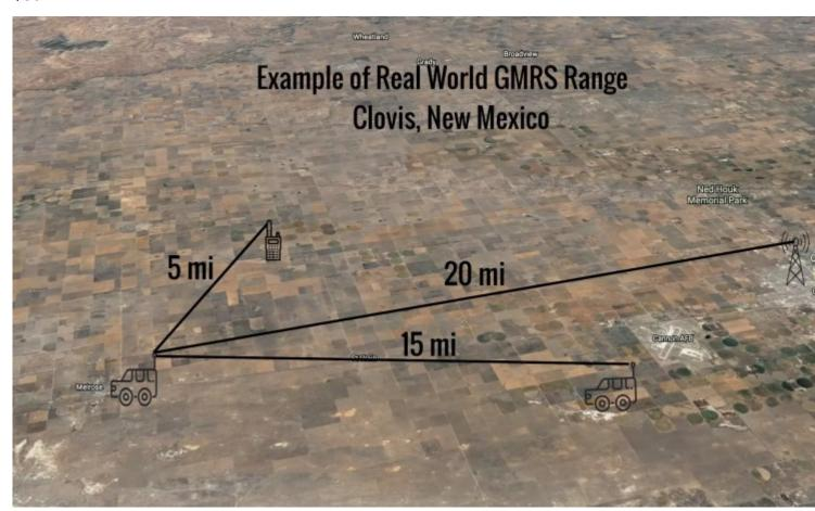
GMRS radios typically provide much longer range than FRS handhelds. Example of real-world GMRS range, level terrain.
