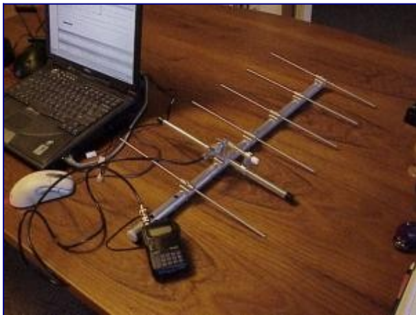
Gene Preston K5GP's 440 MHz yagi and hand-held receiver (used in AM mode.)
