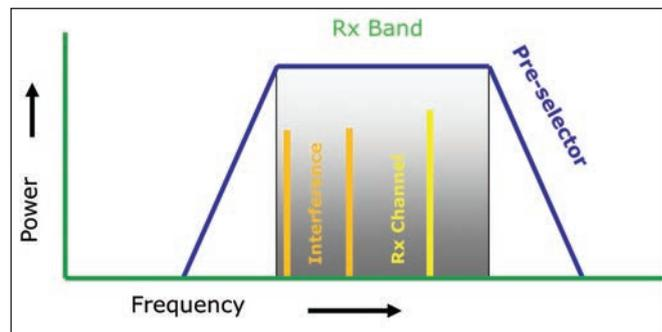
Figure 2. Interfering signals may be off-channel but inband.
