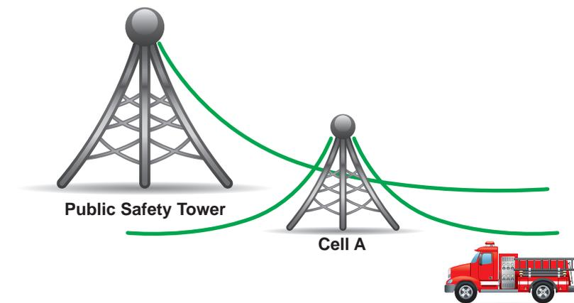
Figure 13. Near-Far problems with cellular and point-to-multi-point transmissions.
