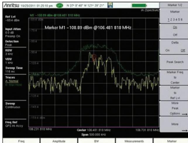
Figure 26. Signal centered on screen with Max-Hold enabled.
