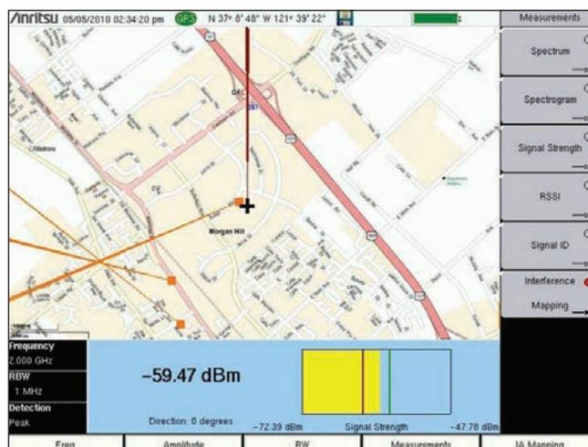
Figure 27. Plotting directions to an interference source on a map.
