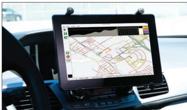
Figure 19. Interference hunt screen capture. Dots shown along drive path are colored according to signal strength.
