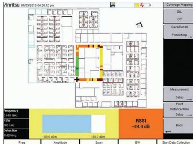
Figure 28. Plotting signal strength to find an interference source.
