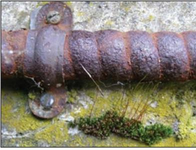
Figure 34. Cleaning up sources of PIM can cure interference problems.
