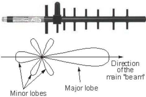
Figure 21. A Yagi antenna and its pattern.
