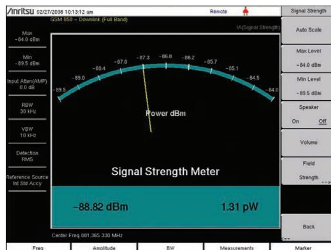
Figure 29. A Signal Strength Meter.
