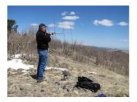
Bob KØNR operates 2m FM using an HT and small Yagi antenna from Aspen Ridge in Colorado. A basic VHF SOTA station is a handheld FM transceiver with a ½-wave telescoping antenna. The standard rubber duck on a handheld transceiver (HT) is generally a poor radiator so using a ½-wave antenna is a huge improvement. Just stuff the HT and antenna in a backpack along with the usual hiking essentials and head for the summit.
