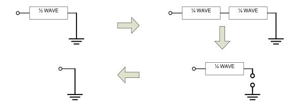
The exception to this is when the terminating impedance is equal to the impedance of the cable. In this case, the cable / impedance combination acts as if the cable was not there irrespective of the length of the cable.
