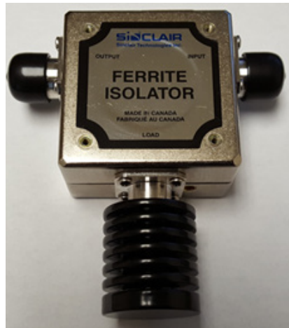
Figure 4: The circulator becomes an isolator when a matched 50-ohm load is added
