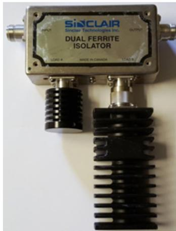
Figure 6a: Dual isolator type “A”
