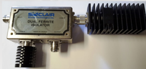
Figure 6b: Dual isolator type “B”
