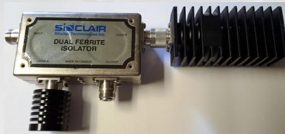
Figure 6b: Dual isolator type “B”
