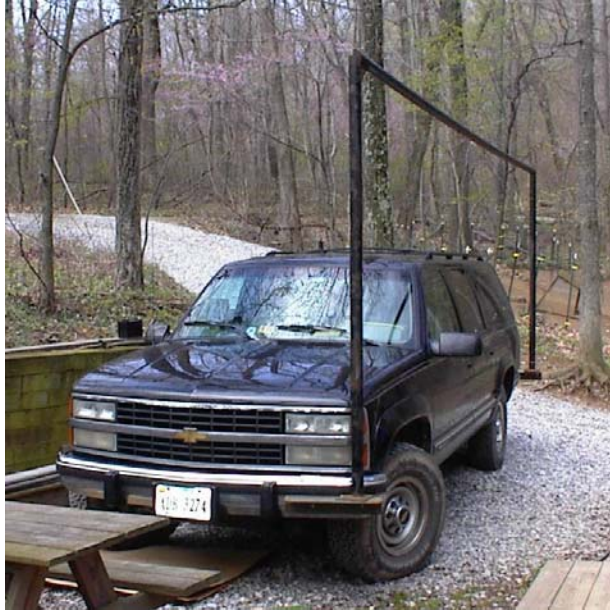
Figure 25: Home-brew HF Mobile NVIS Loop Antenna
